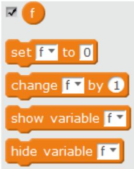
The first two blocks are used to define the variable value and the varied value of the variable. The other two blocks are mostly used for stage creation model.
