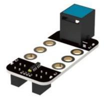
The line follower has 2 sensors which can detect a white surface (within the range of 1-2cm). It works by emitting IR (InfraRed) light and recording how much is reflected back. If a lot is reflected back, it can be deduced it is close to a white surface. If a little is reflected back, it can be deduced that the surface is black, or the sensor is not near a surface.
