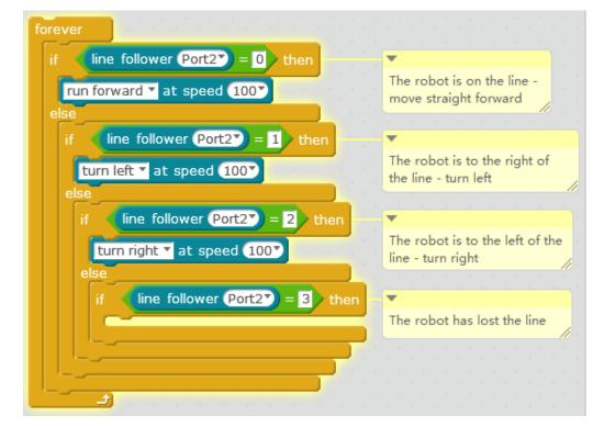
And it doesn't work – the robot often goes off the track. This is because this program is run from the mBlock IDE. Remember it takes time for the signals and commands to be sent from the robot to the computer and back again. In this case, that delay interferes with how the robot performs the line following. We need to upload this program onto the board to reduce this delay. Then the program will work. For the mBot, we use the "mBot program" block, go into Arduino mode and "Upload to Arduino":
