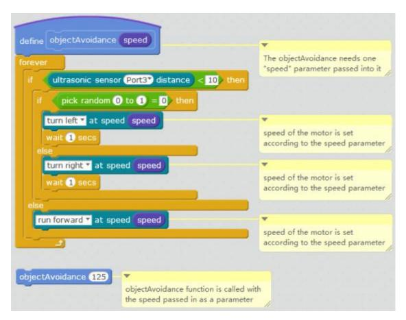
At the bottom you can see the objectAvoidance function is called and it passes in a speed of 125.
