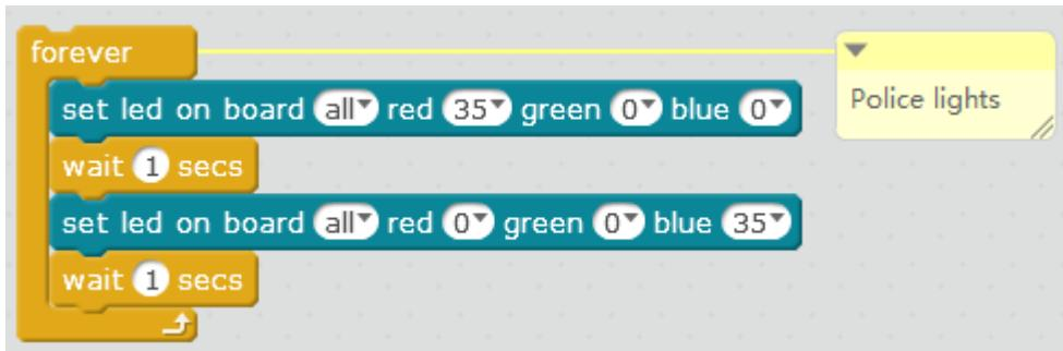
Notice that I need 2 wait blocks – one after the red LED is turned on, and one at the bottom of the loop, where the blue LED is turned on.
