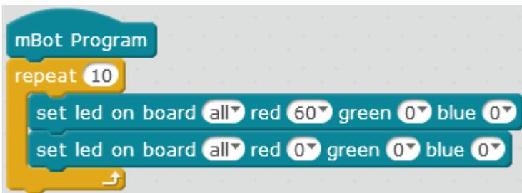
Repeat it for 10 times and the LED light will be turned on and off. You cannot even see the blinking (the script runs in a blink).
