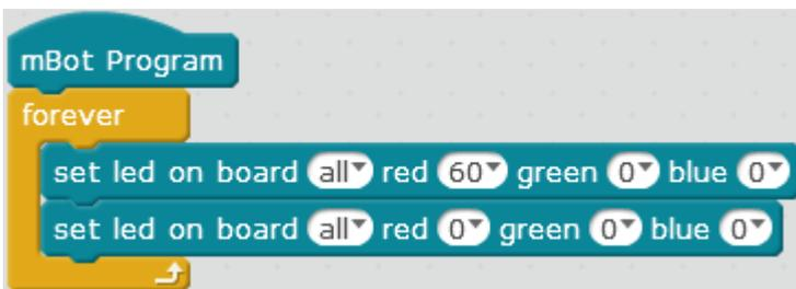
Repeat it for unlimited times and the LED light is kept on (the script runs continually and your eyes cannot capture the blinking).
