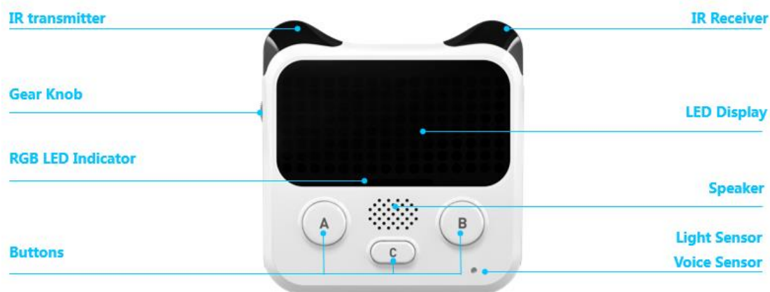
Figure 1 Product Layout of Codey
